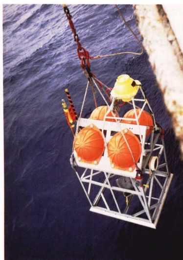
Fig. 2. Outer view of the ocean bottom proton magnetometer being installed.
