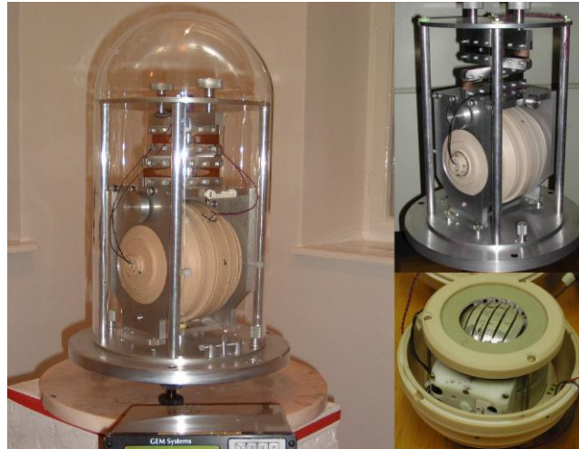
Figure 1: Suspended dIdD with view showing version with housing removed and advanced spherical sensor from GEM.
