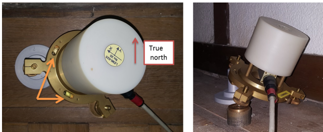
Figure 3. LEMI-025 installed in the Dourbes magnetic observatory. The red arrow indicates the true north direction. The orange arrows highlight the bubble-levels saturation.
