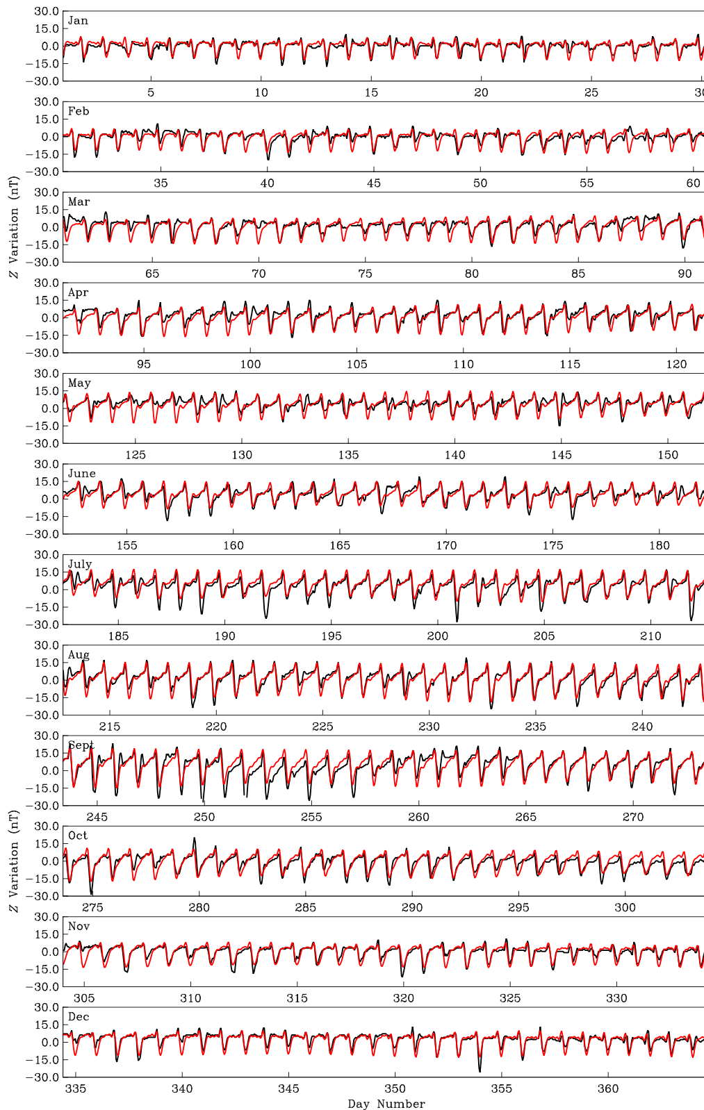
Figure 3. Time-series of HON vertical component Z variation for 2008 (black, Section 2) and a discrete-frequency, synthetic model of long-term average solar-diurnal variation (red, Section 11). A constant average baseline has been subtracted from each window of time.
