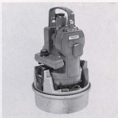
Fig. 14 For packing, the illumination torch slides onto one of the clamps of the container base plate.
