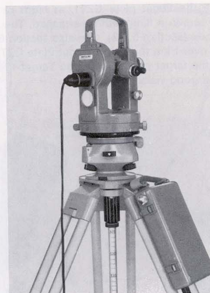
Fig. 15 T1 with Battery Box Illumination Set
