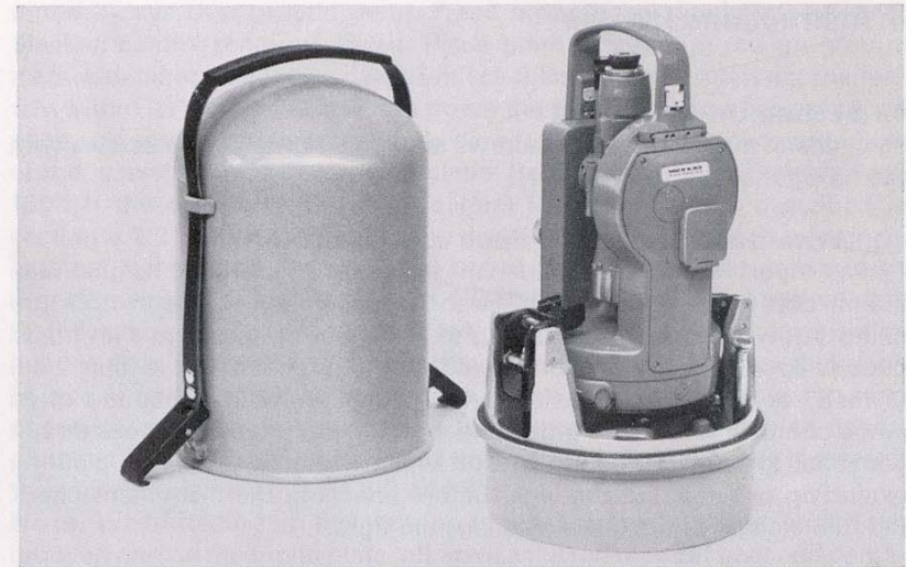
Fig. 4 The Wild T1 and its container. The red mark on the alidade must be over the red dot on the lower plate drive.
